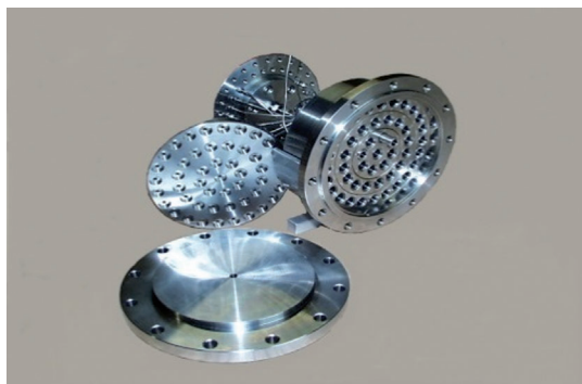
Figure 9. Parallel reactor technology developed by the Schüth group featuring a parallel channel high-throughput reactor with a pressure rating of 50 bar used for methanol synthesis. [59]
